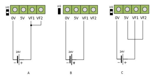
A/ Pi Powered by field 1, which also powers all field supplies
