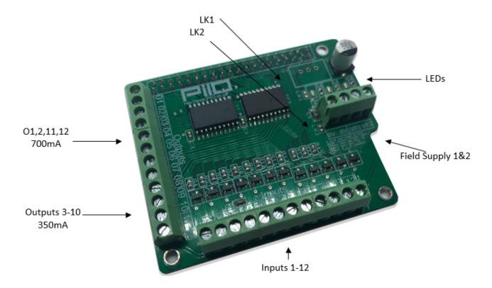
**Note** – This board requires the GPIO extender kit in order to work with the Pi4 B, this raises the height of the board above the ethernet connector.
