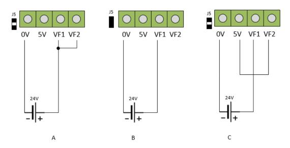
A/ Pi Powered by field 1, which also powers all field supplies
