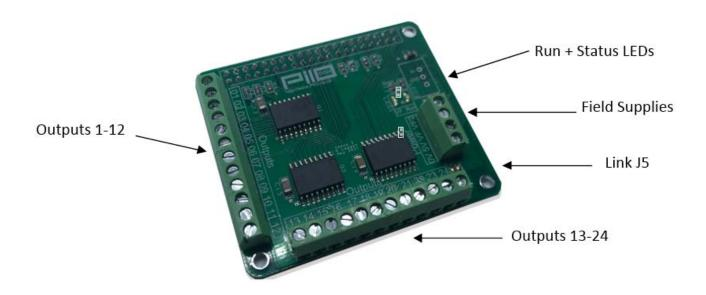
**Note** - PiIO-XXX-H Boards follow the Pi HAT mechanical specification but do not have an onboard device ID EEPROM.
