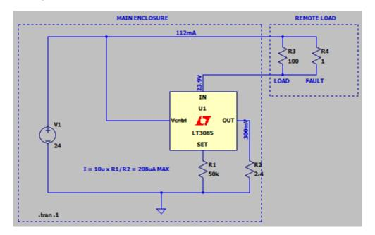
There are a variety of circuits to do this, you can also use discrete NPN transistors as well as using older regulators like the LM317 if you prefer the positive rail to be limited. Here R1 sets the maximum current. The dropout voltage for the LM317 is 1.5-2.5V however so you need to establish that would be acceptable to your design (as it's subtracted off the output voltage).
