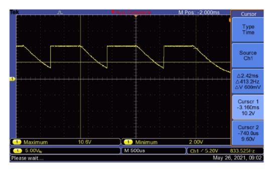
Adding a 1KR Load however solved this issue, it should be noted therefore for fast switching performance the outputs should be loaded.
