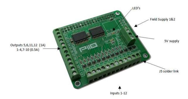
PiIO-XXX-H Boards follow the Pi HAT mechanical specification but do not have an onboard device ID EEPROM.
