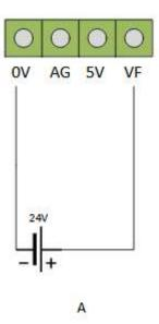
A/ Pi Powered by field supply, which also powers all field supplies
